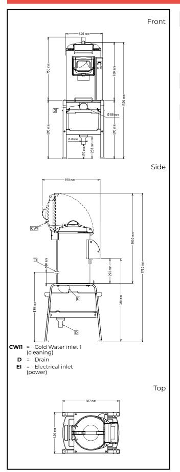
Electric Supply voltage: 603511 (DT15E1) 220-240 V/1N ph/50/60 Hz 200-240/380-440 V/3 603512 (DT15E324) ph/50/60 Hz Electrical power, max: 0.37 kW 0.37 kW **Total Watts:** Capacity: Performance (up to): 240 kg/hour Capacity: 15 litres Key Information: External dimensions, Width: 440 mm External dimensions, 690 mm Depth:
